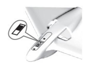
Turn the power switch to off position on both the Shadow Caster and the charger . If either is turned on, the Shadow Caster will not charge.
