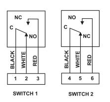
Figure B-7. Switch When Ball Valve is in Fully Open Position
