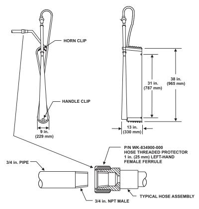
Figure 4-44. Hose Rack Installation
