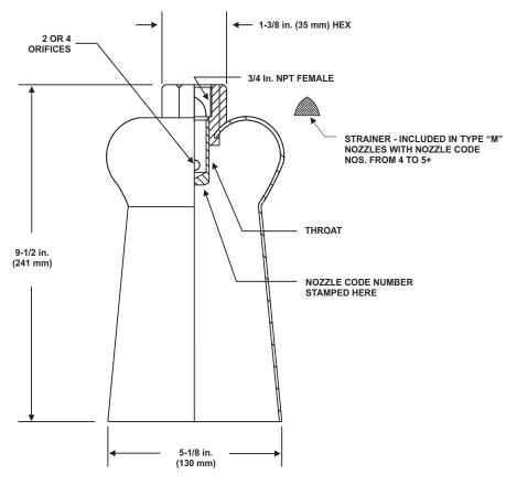
Figure 2-64. Multijet Nozzle, Type M
