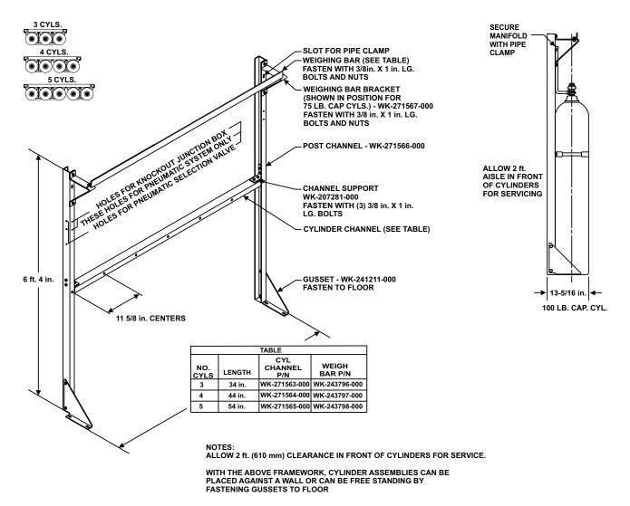
Figure 4-13. Rack Framing -3 to 5 Cylinders (100 lb. Capacity), Single Row
