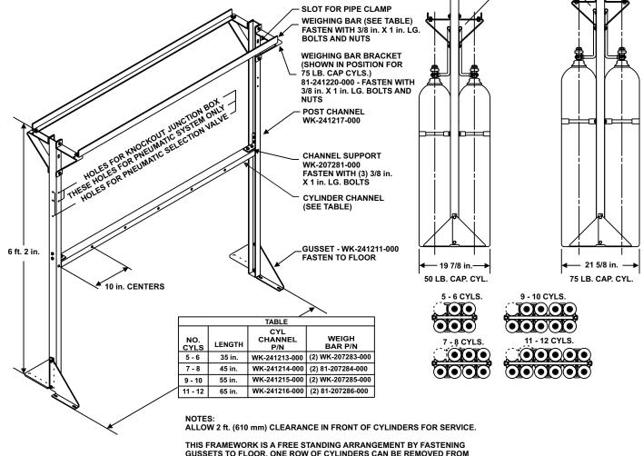
GUSSETS TO FLOOR. ONE ROW OF CYLINDERS CAN BE REMOVED FROM EACH SIDE FOR SERVICING, THEREFORE A 2 ft. (610 mm) AISLE ON EACH SIDE IS REQUIRED.
