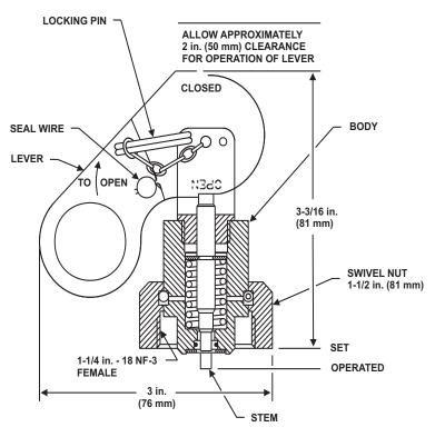
Figure 2-20. Lever-Operated Control Head
