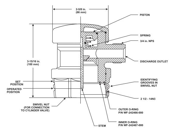
Figure 2-8. Discharge Head, Grooved Nut
