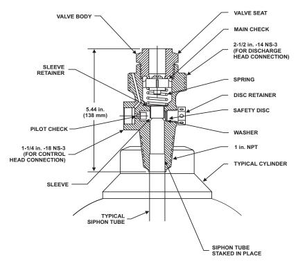
Figure 2-4. 5/8-inch Type "I" Cylinder Valve
