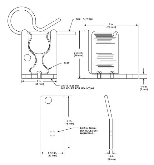
Figure 4-47. Handle and Horn Clips
