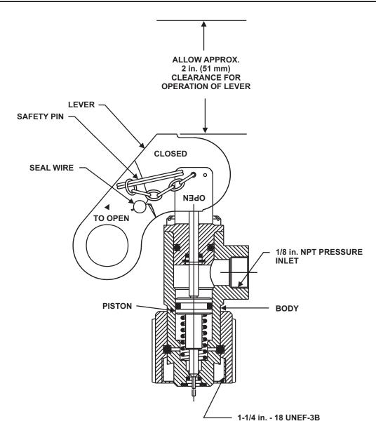
Figure 4-35. Lever and Pressure Operated Control Heads
