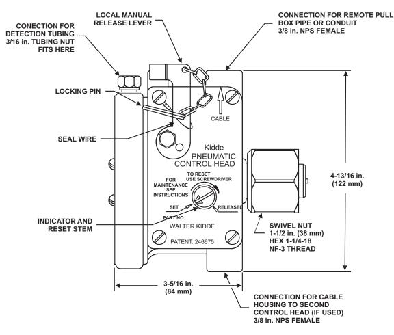
Figure 2-35. Pneumatic Control Head
