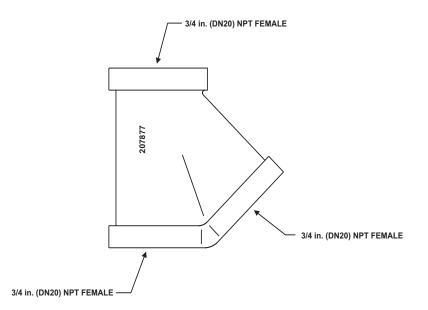
Figure 4-2. Manifold "Y" Fitting
