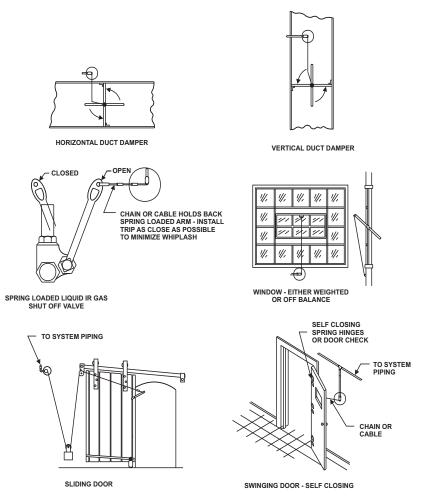
Figure 3-13. Pressure Trip Applications
