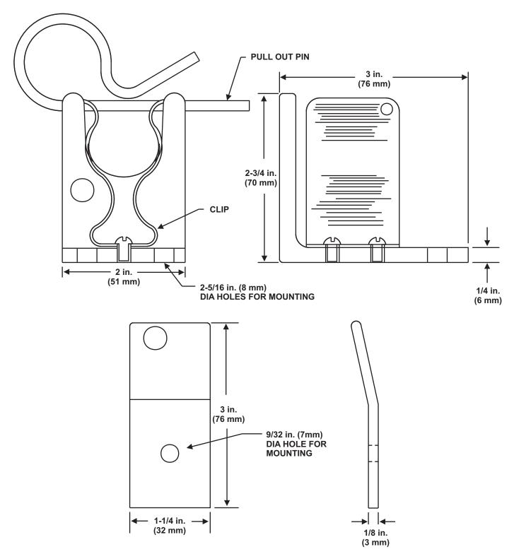
Figure 2-93. Handle and Horn Clips
