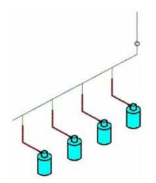
Figure 3-6. Example of an "End" Manifold
