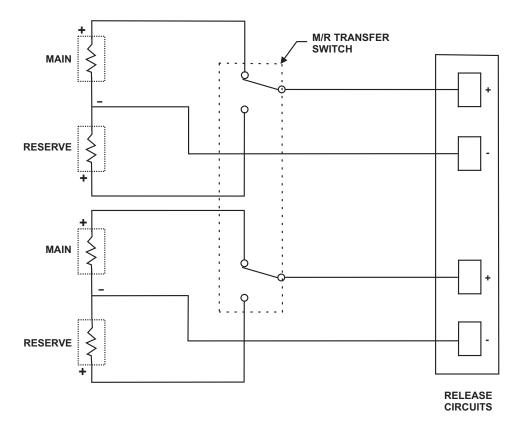
Figure 4-24. Wiring Diagram with Dual Solenoid (Main and Reserve)
