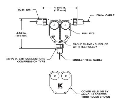
Figure 2-26. Tee Pulley
