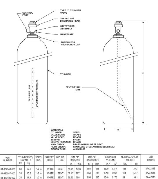
Figure 2-1. 25 through 50 lb. Carbon Dioxide Cylinders, Bent Siphon Tube
