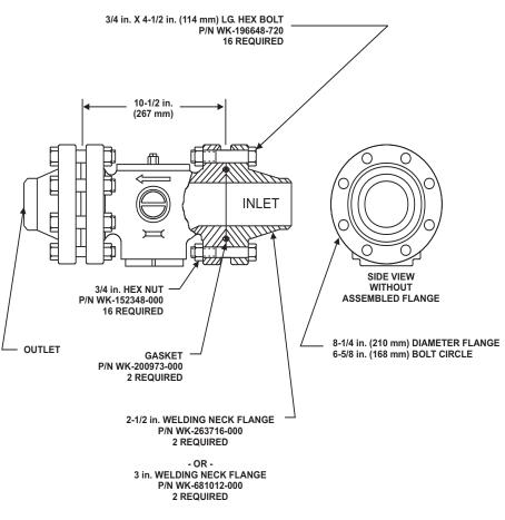
Figure 2-50. Check Valves (2 1/2-inch to 3-inch)
