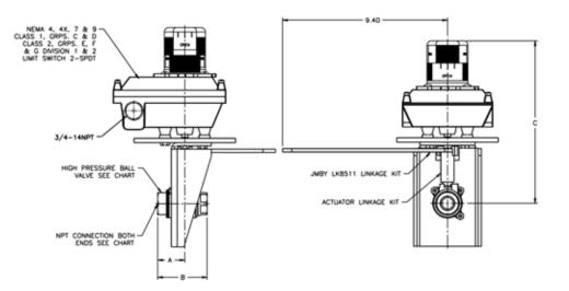
Figure 2-57. Lockout Valve with Explosion Proof Limit Switches
