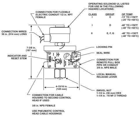
Figure 2-34. Explosion Proof Electric and Cable Operated Control Head
