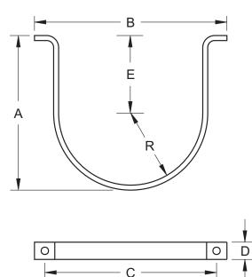
Figure 2-14. Single Cylinder Straps
