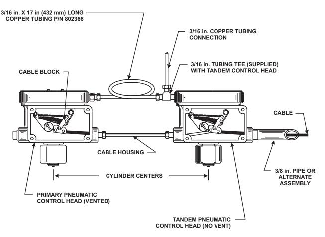
Figure 4-32. Tandem Pneumatic Control Head
