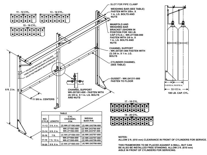
Figure 4-18. Rack Framing - 11 to 20 Cylinders (100 lb. Capacity), Double Row (One Side)
