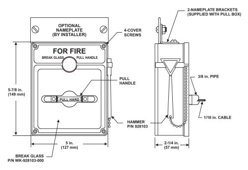
Figure 2-23. Mechanical Pull Box
