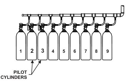
Figure 3-11. Pilot Cylinder Position within Manifold
