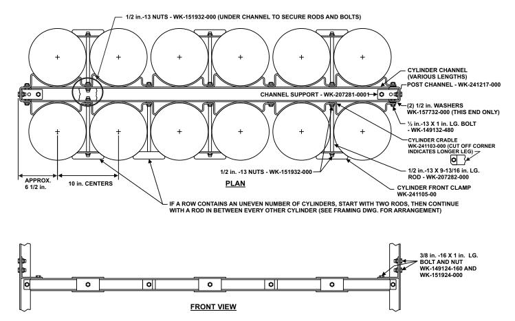
Figure 4-12. Cylinder Racks (50 and 75 lb. Capacity), Double Row (Two Sides)
