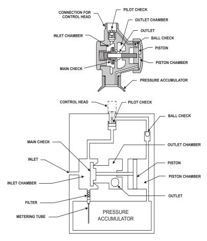
Figure 2-72. Pneumatic Discharge Delay, Detail
