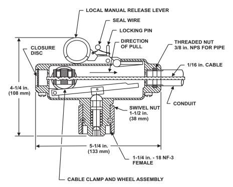
Figure 2-21. Cable-Operated Control Head
