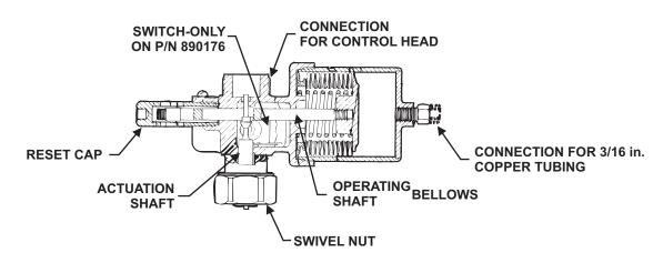
Figure B-3. Pneumatic Transmitter
