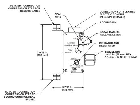
Figure 2-33. Electric and Cable-Operated Control Head
