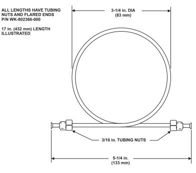
Figure 2-41. 3/16-inch Pneumatic Tubing
