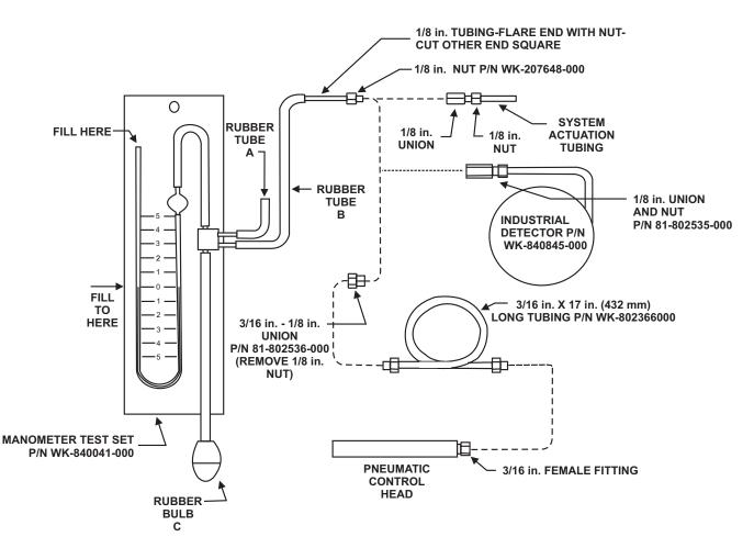
Figure 4-29. Manometer Pneumatic Detection
