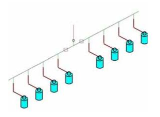
Figure 3-9. Example of a "Main and Reserve" "End" Manifold
