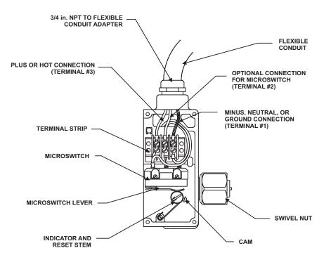
Figure 2-32. Electric Control Head (Cover Removed)
