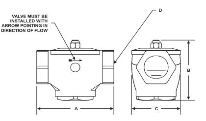
Figure 2-49. Check Valves (1-1/2-inch to 2-inch)
