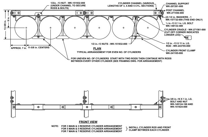
Figure 4-16. Cylinder Racks (100 lb. Capacity), Single Row
