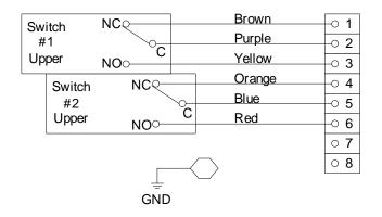
Figure 3-10. Lockout Valve Release Circuit Wiring
