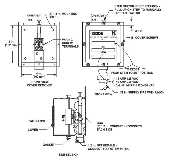
Figure 2-68. Pressure Operated Switch
