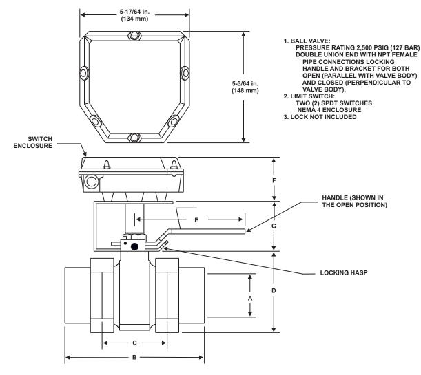
Figure B-6. CO<sub>2</sub> Lockout Valve with Limit Switch
