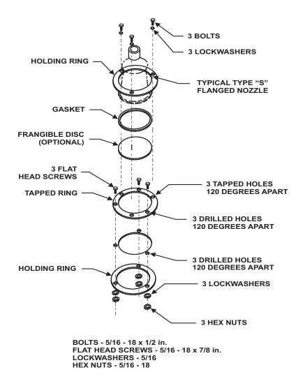
Figure 2-62. Flanged Nozzle Mounting Kit (Duct or Enclosure Mounting)
