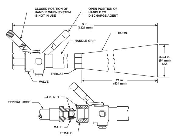
Figure 2-92. Horn and Valve Assembly
