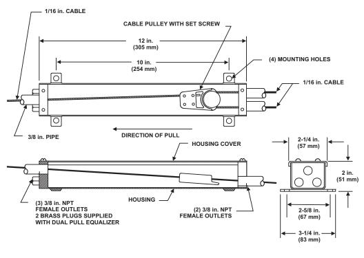
USE 3/32 in. HEX KEY FOR CABLE PULLEY SET SCREWS
