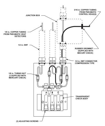
Figure B-2. 3-Well Mercury Check - Installation Detail
