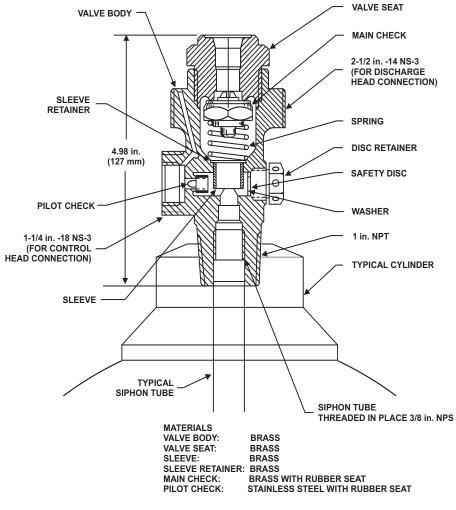
Figure 2-3. I/2-inch Type "I" Cylinder Valve
