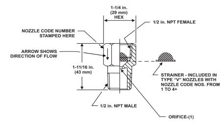
Figure 2-65. Vent Nozzle, Type V
