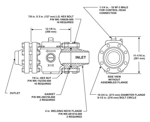
Figure 2-53. Directional (Stop) Valve (4-inch)
