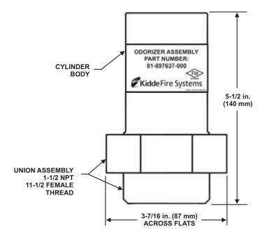
Figure B-9. Odorizer Protective Housing
