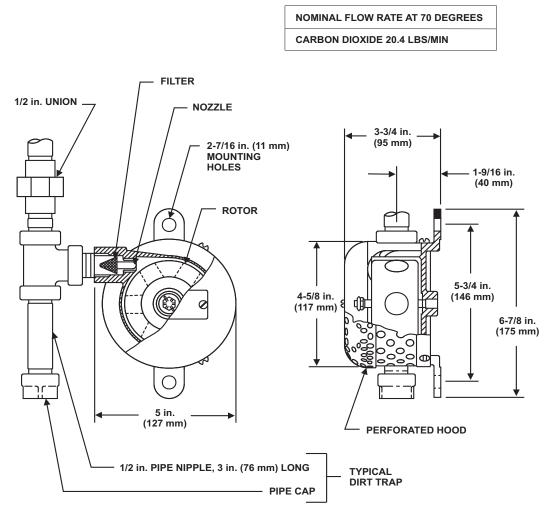
Figure 2-74. Pressure Operated Siren
