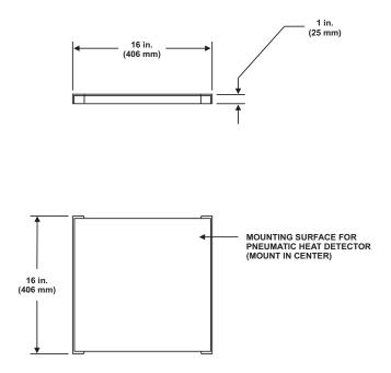
Figure 2-39. Heat Collector
