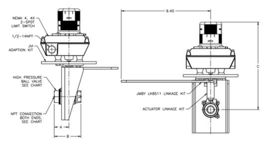
Figure 2-56. Lockout Valves with Limit Switches
