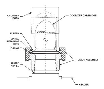
Figure B-11. Odorizer Installation
