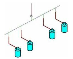
Figure 3-7. Example of a "Center" Manifold
