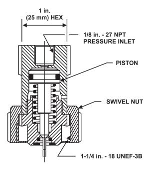
Figure 4-34. Pressure Operated Control Heads
