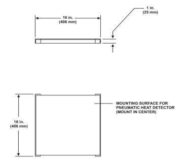
Figure 4-30. Heat Collector
