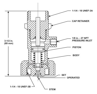
Figure 2-44. Stackable Pressure Operated Control Head
