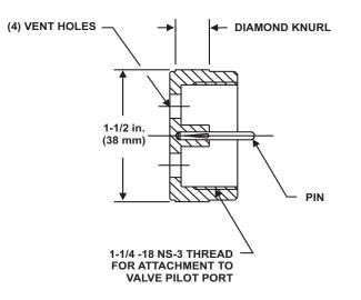
Figure 2-81. Blow-Off Fixture
