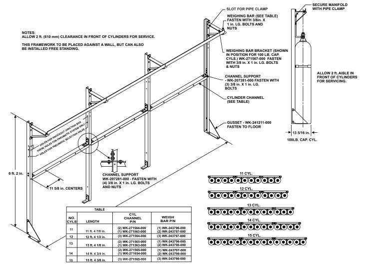
Figure 4-15. Rack Framing - 11 to 15 Cylinders (100 lb. Capacity), Single Row
