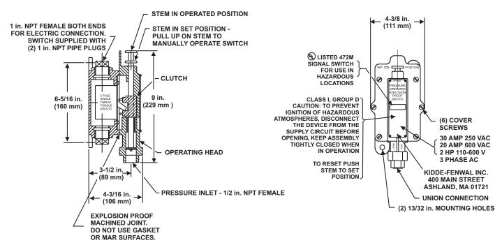
Figure 2-69. Pressure Operated Switch, Explosion Proof
