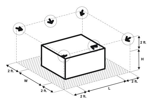
Figure 3-5. Nozzle Placement Example
