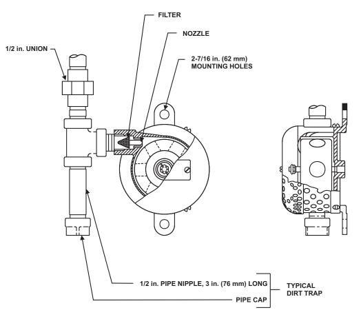
Figure 4-39. Pressure Operated Siren
