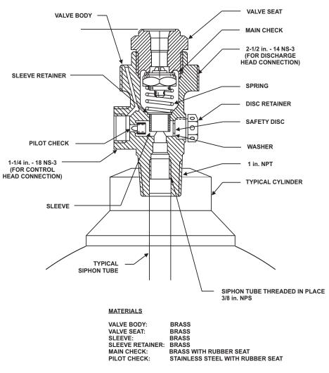
Figure 7-1. I/2-inch Type "I" Cylinder Valve
