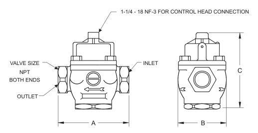
Figure 2-51. Directional (Stop) Valves (1/2-inch through 2-inch)
