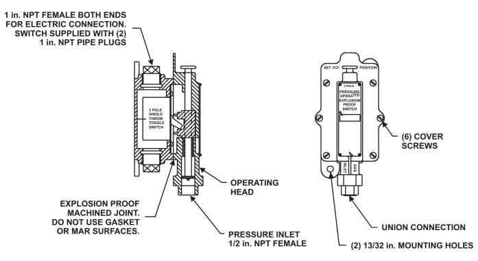
Figure 4-37. Pressure Operated Switches, Explosion Proof
