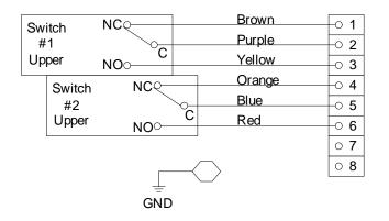
Figure 4-22. Wiring Diagram for Lockout Valve when Ball Valve is in Fully Open Position
