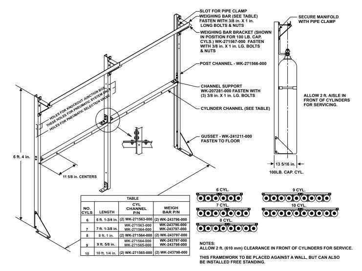
Figure 4-14. Rack Framing - 6 to 10 Cylinders (100 lb. Capacity), Single Row
