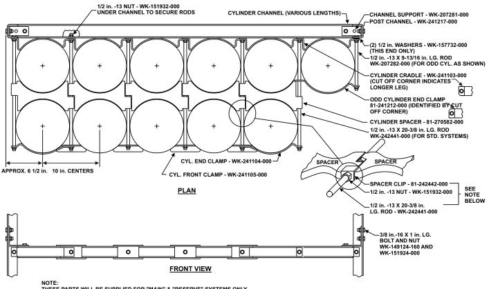
THESE PARTS WILL BE SUPPLIED FOR "MAIN" & "RESERVE" SYSTEMS ONLY. THE PARTS WILL SECURE THE REAR ROW "RESERVE" CYLS. WHEN THE FRONT ROW "MAIN" CYLS. ARE REMOVED FOR RECHARGING. USE ONE SPACER CLIP PER ROD, AND SECURE WITH NUT SUPPLIED.
