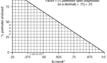
Figure 3-4. Partial Enclosure Flow Rate Reduction\*
