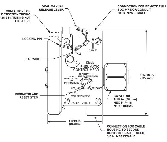
Figure B-4. Pneumatic Control Head (1-inch, 40-second)
