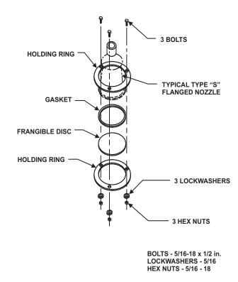
Figure 2-61. Flanged Nozzle Mounting Kit (Orifice Protection Only)
