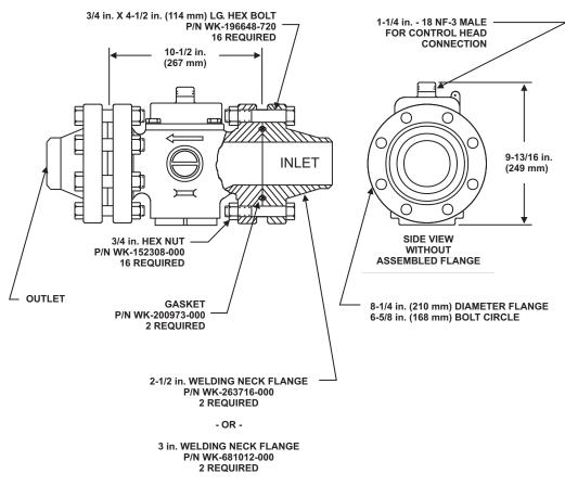
Figure 2-52. Directional (Stop) Valves (2-1/2-inch and 3-inch)
