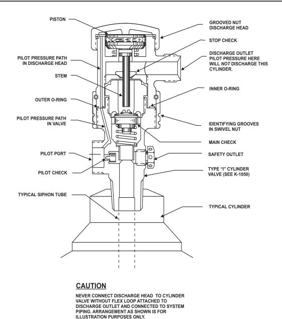
Figure 2-9. Installation of Grooved Nut Discharge Head to Cylinder Valve
