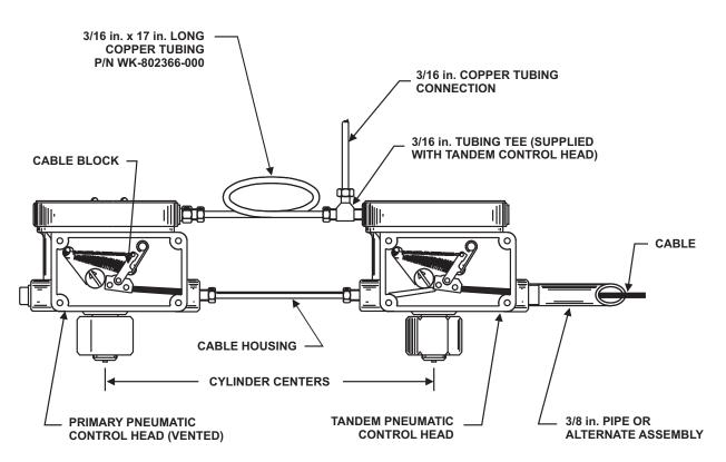
Figure 2-36. Tandem Pneumatic Control Head
