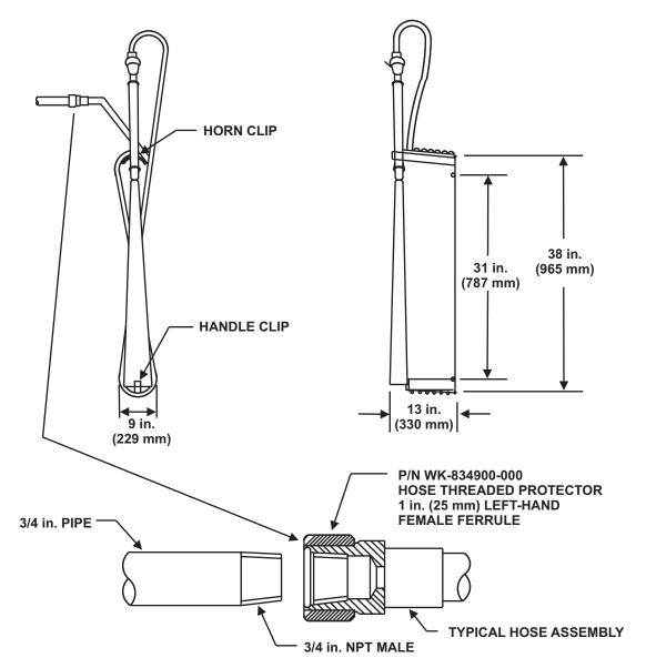
Figure 2-90. Hose-to-Pipe Rack Connection
