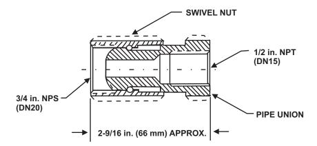
Figure 4-21. Swivel Adapter to Piping
