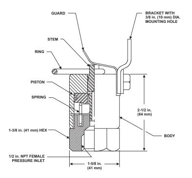
Figure 2-70. Pressure Operated Trip
