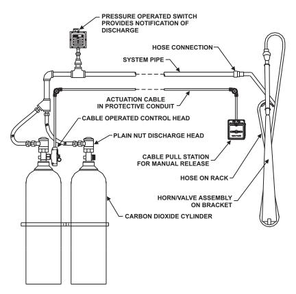
Figure 3-14. Typical Hand Hose Line System with Rack
