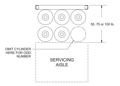
Figure 2-18. Multiple Cylinder Mounting, Arrangement C
