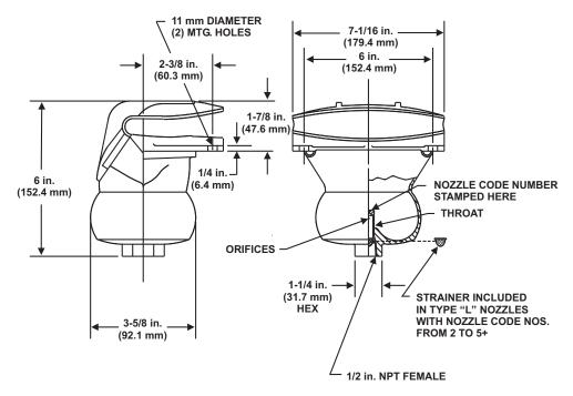
Figure 2-67. Multijet Nozzle, Type L
