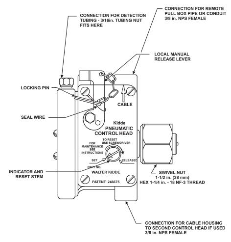
Figure 4-31. Pneumatic Control Head
