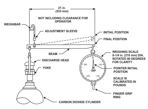
Figure 6-2. Carbon Dioxide Cylinder Weighing Scale
