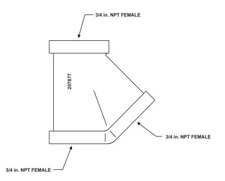
Figure 2-13. Manifold "Y" Fitting
