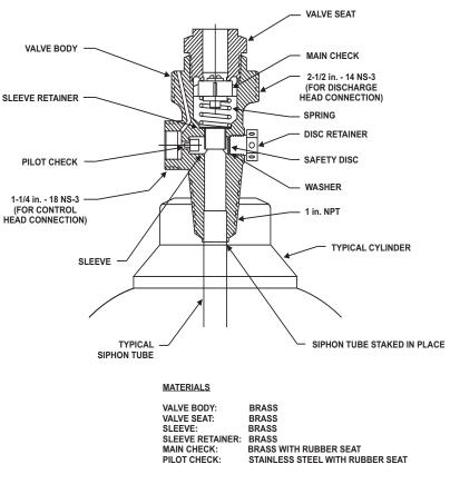
Figure 7-2. 5/8-inch Type "I" Cylinder Valve
