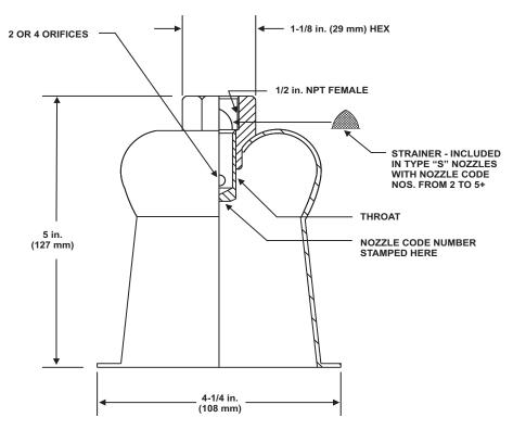
Figure 2-60. Multijet Nozzle, Type S Flanged
