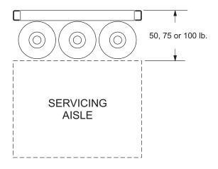
Figure 2-16. Multiple Cylinder Mounting, Arrangement A
