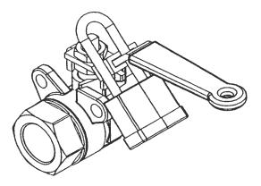
Figure 2-55. Lockout Valves with Lock
