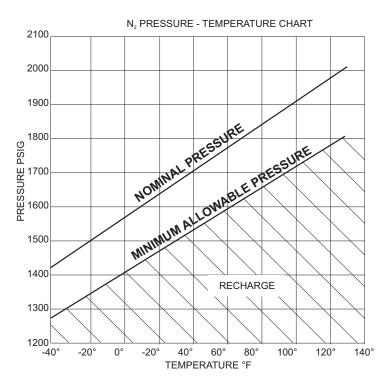
Figure 6-1. Nitrogen Temperature vs. Pressure Data
