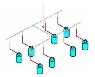
Figure 3-8. Example of an "H" Manifold
