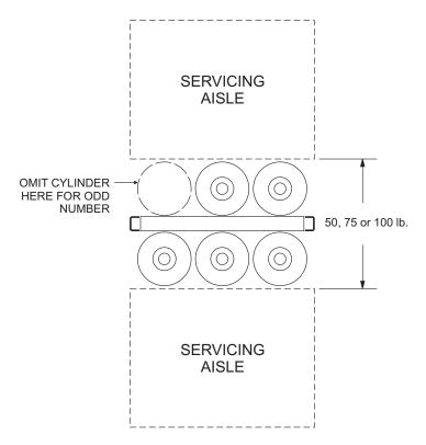
Figure 2-17. Multiple Cylinder Mounting, Arrangement B
