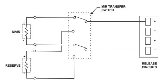
Figure 4-23. Wiring Diagram with Single Solenoid (Main and Reserve)
