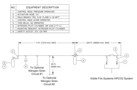
Figure 3-12. Typical Actuation Arrangement Using In-line Discharge Delay
