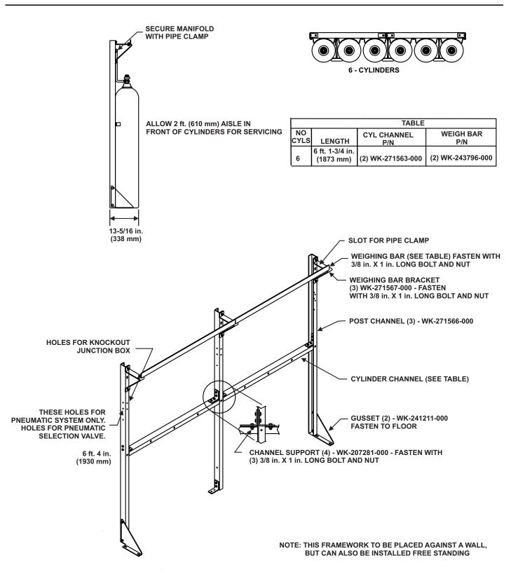
Figure 2-19. Cylinder Rack and Framing, Example Arrangement
