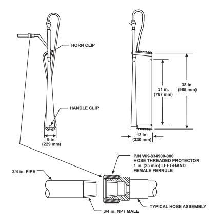
Figure 4-43. Hose Reel Installation
