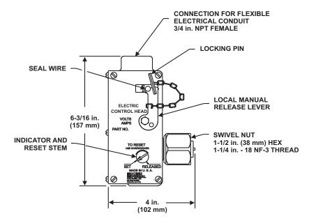
Figure 2-31. Electric Control Head
