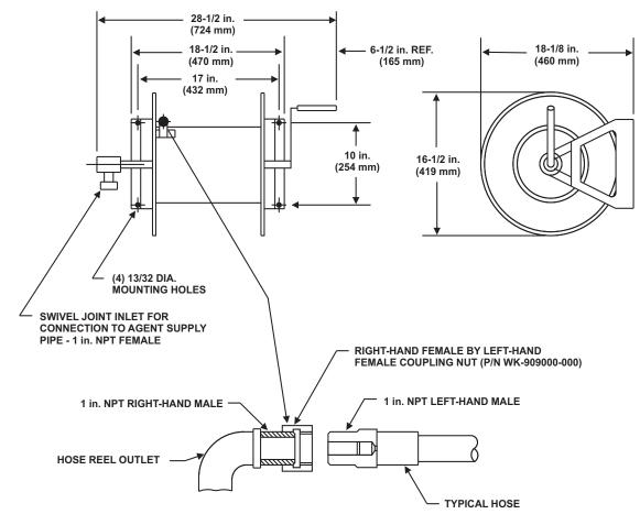
Figure 2-89. Hose-to-Hose Reel Connection
