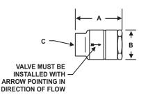
Figure 2-48. Check Valves (1/2-inch to 1-1/4-inch)
