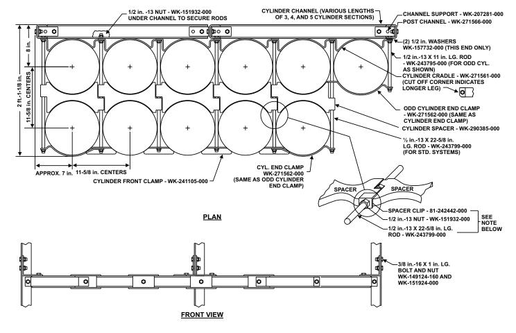
NOTE: THESE PARTS WILL BE SUPPLIED FOR "MAIN" AND "RESERVE" SYSTEMS ONLY. THE PARTS WILL SECURE THE REAR ROW "RESERVE" CYLS. WHEN THE FRONT ROW "MAIN" CYLINDERS ARE REMOVED FOR RECHARGING. USE ONE SPACER CLIP PER ROD, AND SECURE WITH NUT SUPPLIED.
