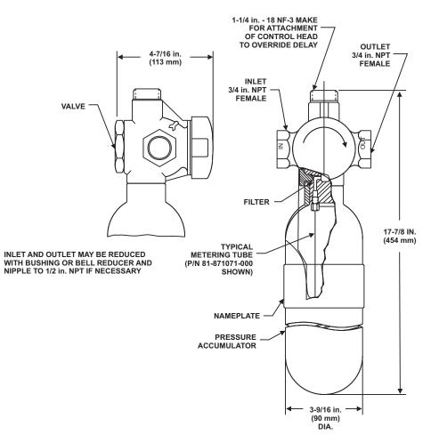
Figure 2-71. Pneumatic Discharge Delay
