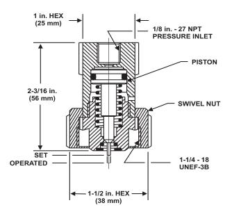
Figure 2-42. Pressure Operated Control Head
