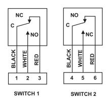
SWITCH 1 IS CLOSED SWITCH 2 IS OPEN
