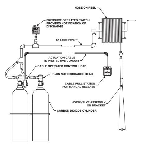
Figure 3-15. Typical Hand Hose Line System with Reel
