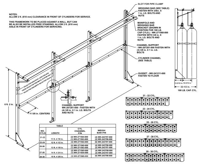
Figure 4-19. Rack Framing - 21 to 30 Cylinders (100 lb. Capacity), Double Row (One Side)
