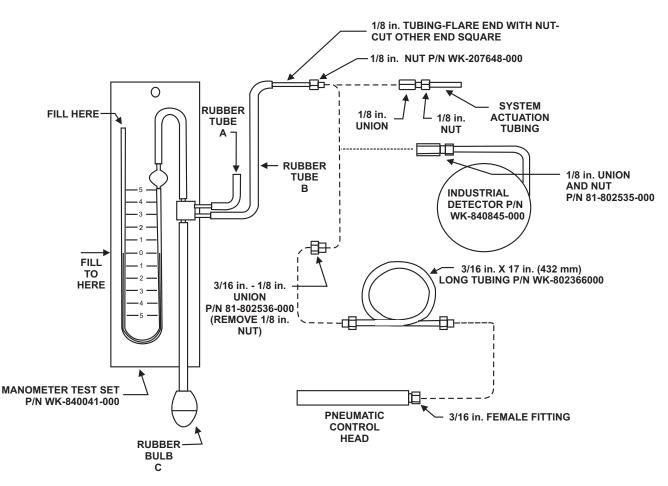
Figure 6-3. Manometer Pneumatic Detection
