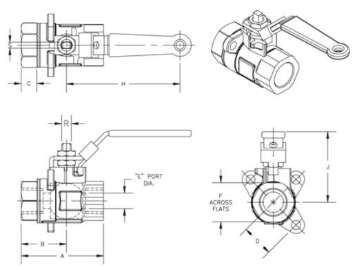
Figure 2-54. Lockout Valves without Limit Switches
