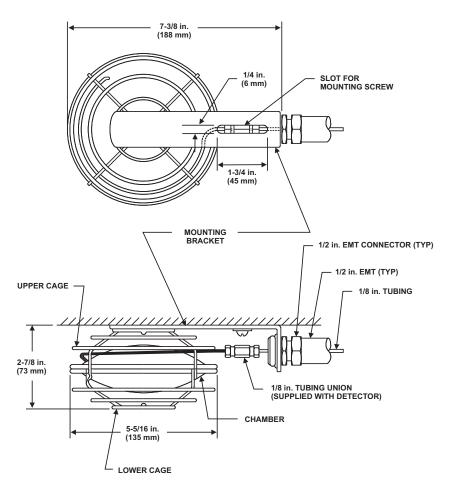
Figure 2-38. Heat Actuated Detector (HAD), Industrial
