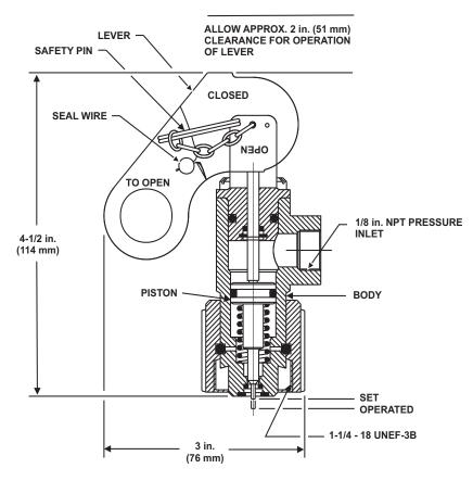
Figure 2-43. Lever and Pressure Operated Control Head
