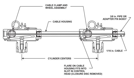
Figure 2-22. Cable-Operated Control Heads in Tandem
