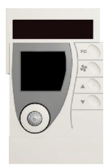
The RPW414-FTL-902-ALC is a solar-powered, self-learning room control module.
