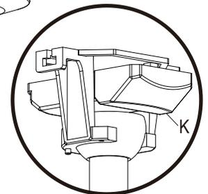
Receiver (K) correctly positioned in mounting bracket.
