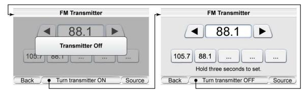
The FM transmitter is turned ON and OFF with the center footer button. The frequency is changed by pressing the arrow left (smaller number) and arrow right (for larger number) buttons. Frequency cannot be changed when the FM antenna is turned off. When the transmitter is turned off all of the buttons and the current frequency are grayed out and the message "Transmitter OFF" is centered on the screen. The default setting is the FM Transmitter Off.
