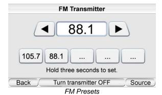
The six preset buttons on the bottom of the screen are used to save the current FM frequency and jump to a saved frequency. By default, all of the buttons display three periods. Pressing and holding a preset button for three seconds saves the current FM frequency, makes a button press sound (a second time), and displays the frequency as the button label.
