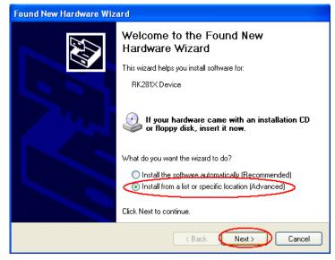
Select "Include this location in the search", and navigate to the following folder "RK3188 Android Upgrade Tool" - "30xxDriver" > "x86" > "XP" on the CD ROM, then click "OK". The system will detect and install the driver automatically, finally click "Finish", see the pictures as below:
