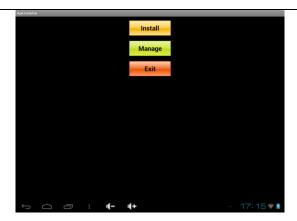
Install: Tap "Install" to enter into the APK installer interface. Files can be put into Internal Memory and RF card
