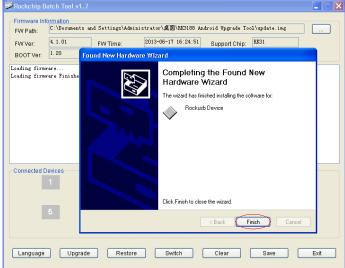
After successful driver installed, Release the "Volume-" key after icon labeled "1" has turned green in the RKBatchTool, see the picture as below:
