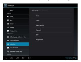
Set unlock pattern, For the screen saver password. Enter the settings interface to click security -screen lock -then click [Pattern] According to prompt settings as Pic
