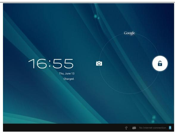
**Power Saving Mode and Locked Mode:** Pressing the "POWER" key when the Tablet PC is in use will make the system enter into SLEEP power save and locked mode. Pressing the "POWER" key or tapping the touch screen for 3 seconds, will return the system to locked mode within 1 second.
