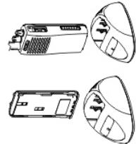
Slide the battery pack or transceiver with a battery pack into the charger. Make sure the battery pack contacts are in contact with the charging terminals. The charger LED turns red and charging begins.
