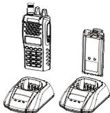
Insert the battery or the radio to be charged into the charger slot.
