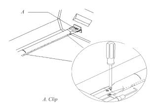
If flame is yellow (not enough air), turn air shutter adjustment screw counterclockwise. If flame is noisy or lifts away from burner (too much air), turn air shutter adjustment screw clockwise.
