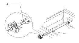
A. Burner/orifice connection
