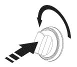
**IMPORTANT:** If the rotisserie burner does not light immediately, turn the rotisserie burner control knob to OFF and wait 5 minutes before relighting.
