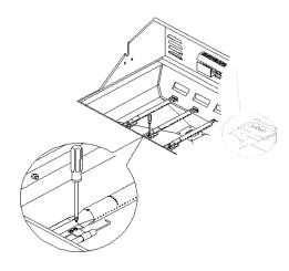
3. Use a 6 mm socket and wrench or 6 mm nut driver to remove the brass orifice from the end of gas valve. The main NG burner orifice is located behind the LP orifice, so no additional orifice needs to be installed.
