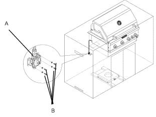
A. Natural gas pressure regulator B. Four 5/32" x 10 mm truss head screws
