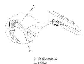
NT: Check that the crifica is properly install
