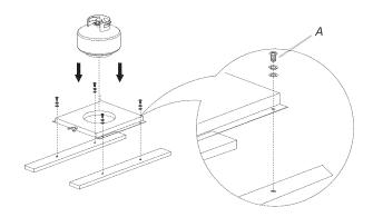
A. Four 5/32" x 10 mm truss head screws
