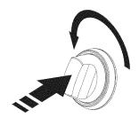
3. When the rotisserie burner lights, continue to hold the knob in for another 10 seconds, then release the knob and burner will stay lit. You will hear the "snapping" sound of the spark until the knob is released.
