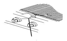
5. Push in and turn the burner knob to IGNITE/HI for the burner closest to the lit match. The burner will light immediately. When burner is lit, turn knob to desired setting.
