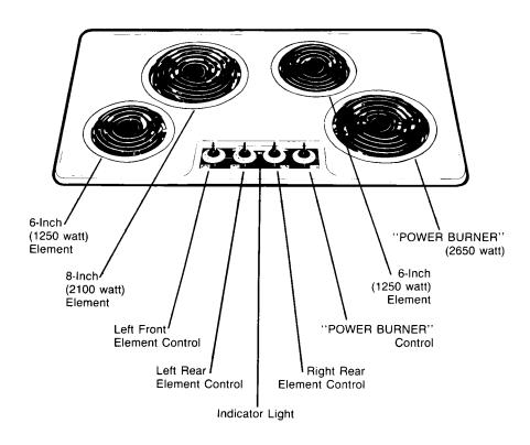
The control knobs for each element have infinite positions ranging from "HI" for highest level of heat available to "LO" for simmer or the lowest heat. There are no fixed positions between "HI" and "LO". You may turn the control knobs in any direction, to any of the settings indicated, or to any position in between.
