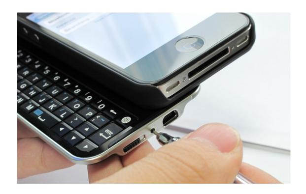
Then the Bluetooth signal light on the left top of the keyboard will be on
