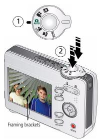
Press the Shutter button halfway to focus and set exposure.
