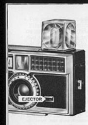
The cube revolves one quarter turn as pressure is removed from the shutter release after making an exposure, thus providing flash for 4 successive exposures if a fresh cube is in place. To use a partially used cube, insert the cube with a fresh bulb forward, keeping in mind the clockwise rotation of the cube to bring succeeding fresh bulbs to the frontal firing position. The cube can also be rotated clockwise (arrow on top of the camera) by hand to position a bulb for firing.
