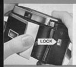
Open the back of the camera by sliding up the LOCK button and swinging out the hinged cover.
