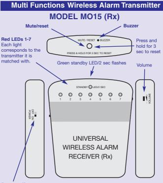
Power off - on Please do not use on/off switch to reset alarm. This will damage the microprocessor.
