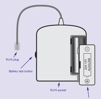
Please observe correct polarity. Contacts clean and battery not loose inside compartment. Pull metal contact to make good connection. Use only 23A 12V Alkaline battery.
