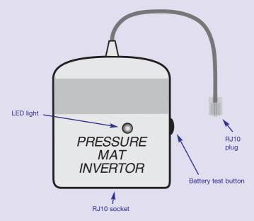
Please plug in the inverter wire between the Pressure-Mat and the transmitter. Battery test: press the button, LED will glow. If LED does not glow then change the battery.
