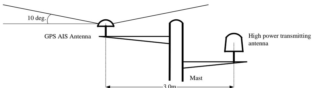
Figure 20 Recommended GPS antenna installation
