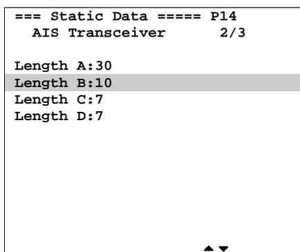
The **AIS transceiver entry** specifies the antenna location for the mobile station's internal GPS receiver.
