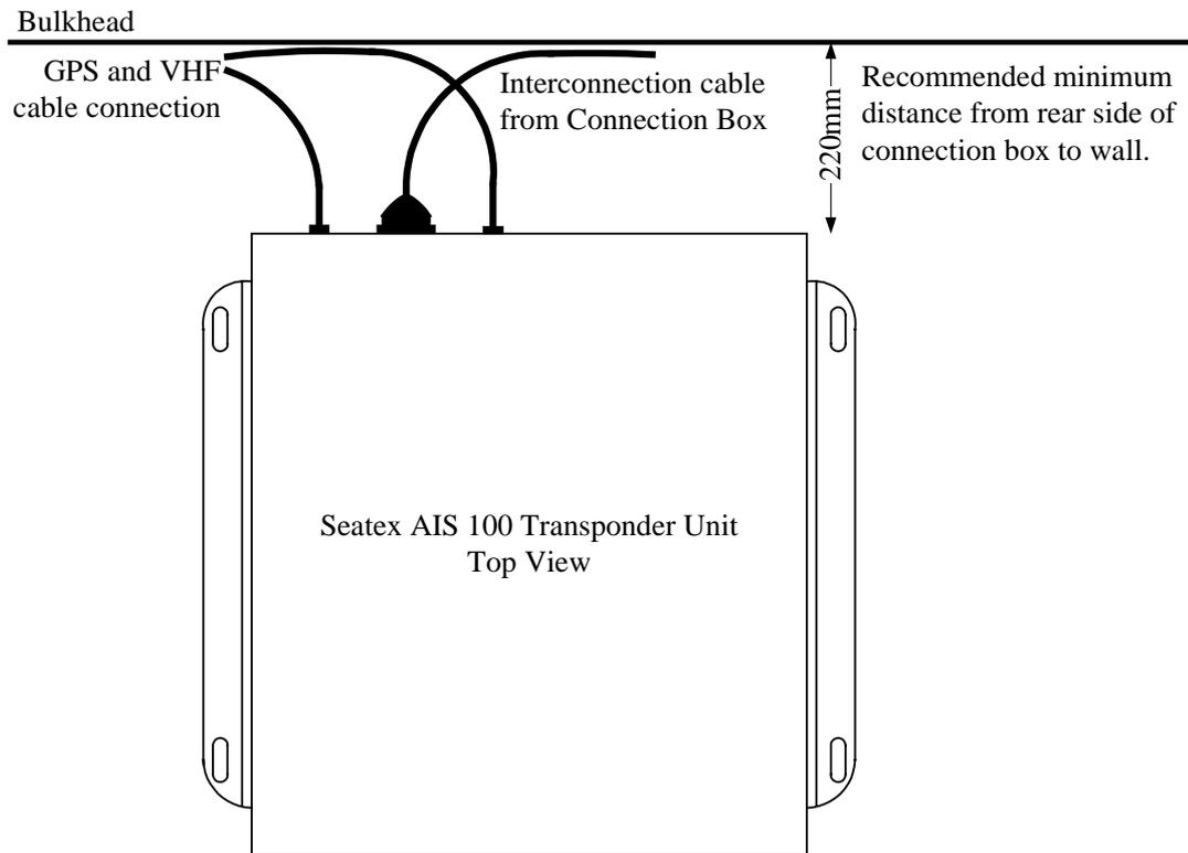
Figure 11 Recommended free space to rear side of mobile station
