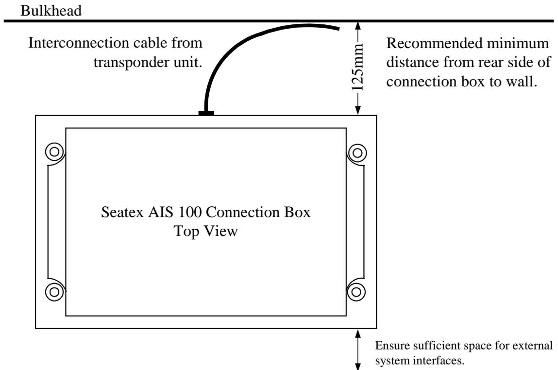
Figure 14 Recommended free space to rear side of connection box
