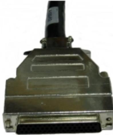
Figure 15 The 50-pin plug
