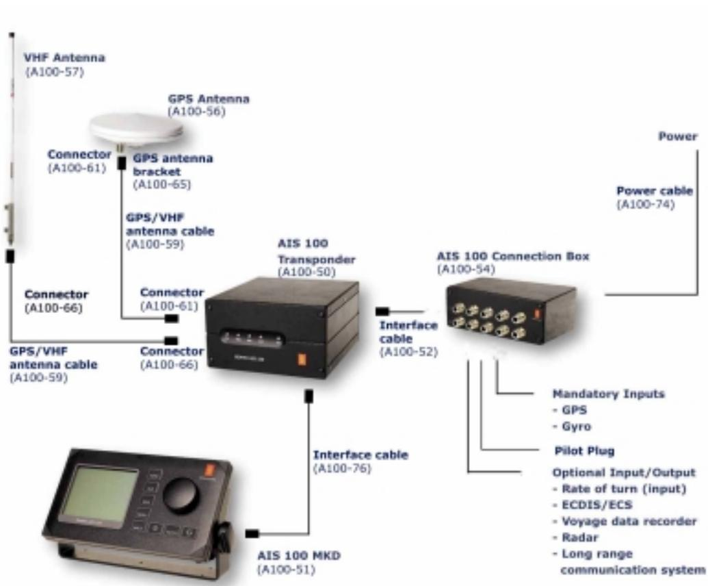
Figure 2 AIS 100 system components
