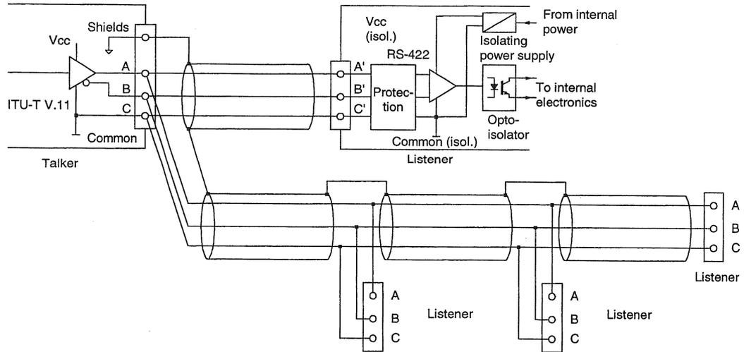
Figure 16 Talker and listener cabling – data/shield
