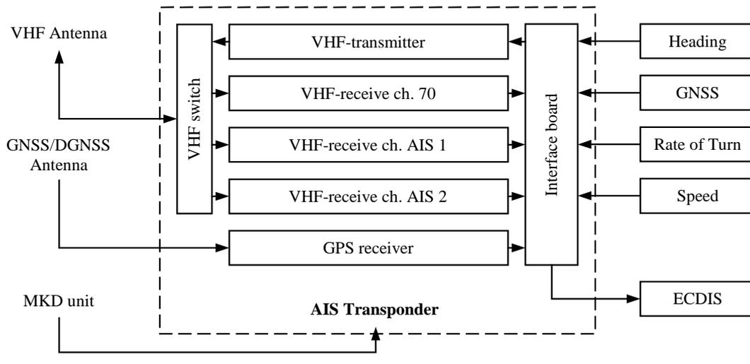
Figure 22 Interfaces to the Seatex AIS 100 mobile station
