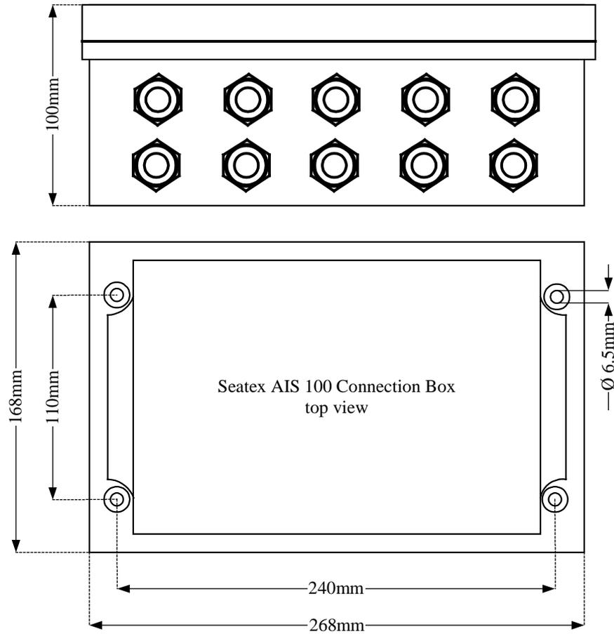
*Figure 6 Connection box dimensions*
