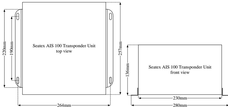
Figure 5 Mobile station dimensions
