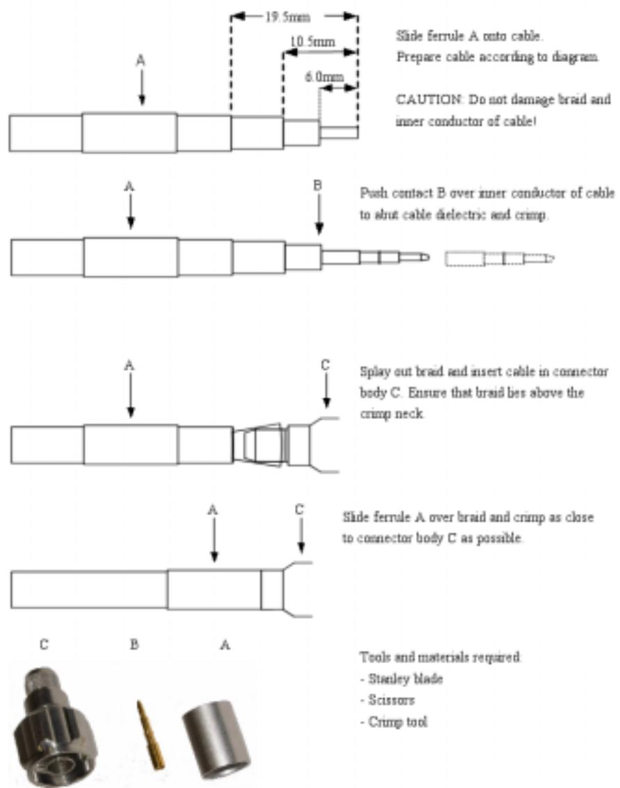
Figure 19 VHF and GPS antenna cable connector termination
