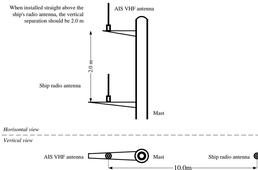
Figure 18 Recommended VHF antenna installation
