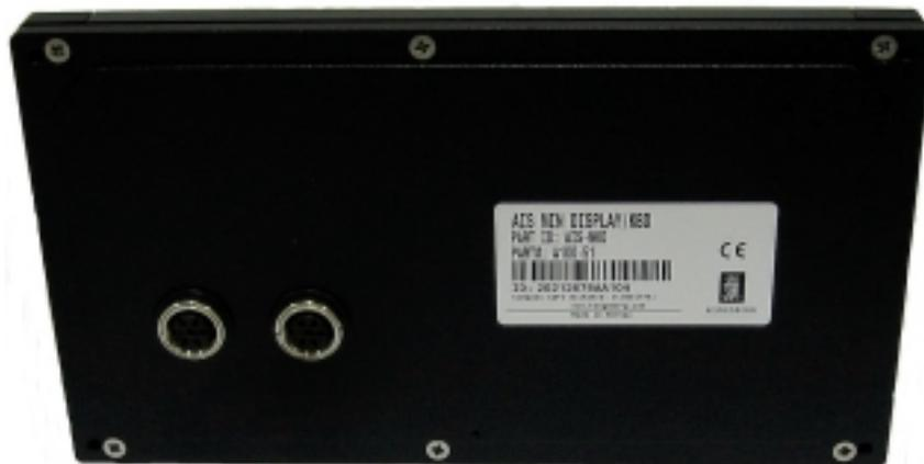
*Figure 9 Rear side of the MKD unit and interconnection plug*
