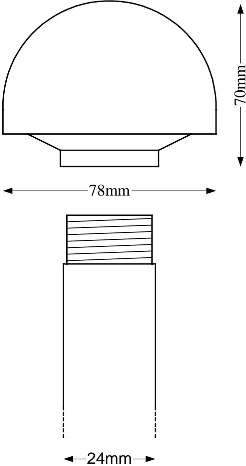
*Figure 8 GPS antenna and pole dimensions*
