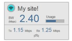
**BW** indicates the bandwidth resource allocated to the local radio site. The **Usage** bar indicates the instantaneous usage of the bandwidth resource.
