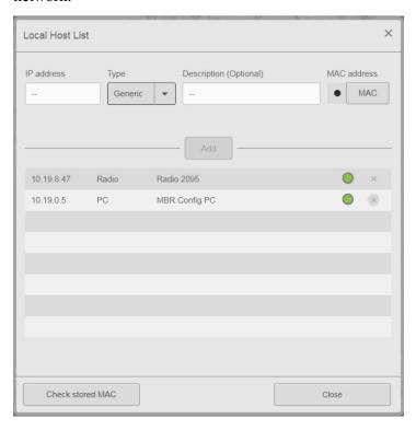
7 Type the IP address of the equipment you want to connect. Select type of equipment from the **Type** list. Type a description of the equipment for identification purposes.
