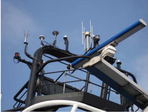
Figure 2 Bad antenna location, typically masking situation
