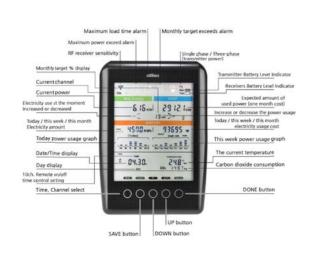
The top section shows Radio Icon, Channel number (1-10), 4- different Alarm Display and Battery power strength display for transmitter and receiver each.
