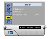
Move the joystick up or down to select the "Position", then press the joystick to select items.
