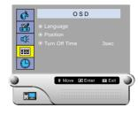
2 Move the joystick up or down to select the "Turn Off Time", then move the joystick left or right to select the seconds you want. The time ranges from 3 to 60seconds.
