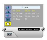
After the hour is entered, press the joystick (at this point the minutes digits will be blinked).
