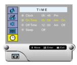
Press the joystick again (the hours digits will be blinked). Move the joystick up or down repeatedly until the correct hour appears.
