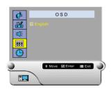
Press the **Menu** button. Move the joystick up or down to select the "OSD", then press the joystick.
