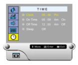
Press the joystick again (the hours digits will be blinked). Move the joystick up or down repeatedly until the correct hour appears.
