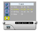
After selecting the correct minutes, press the joystick (the Am / Pm digits will be blinked). Move the joystick up or down to select the "Am" or "Pm".
