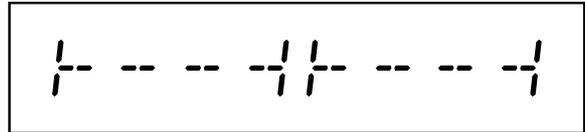
The above display indicates an equal balance between the left and right speakers. To shift the balance to the right, press the "+" (>) button. To shift the balance to the left, press the "-" (<) button. Note you must make the adjustments while the balance setting appears on the front panel display.
