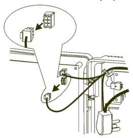
*If the part number of the device is 8602000-xxx*, use the following illustration to locate the connection. Then, disconnect the battery charger board from the mainboard of the device. To do this, press the clip on the
