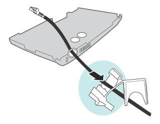
2. Close the top and bottom halves of the clip together and then insert that assembly through the hole in the base.
