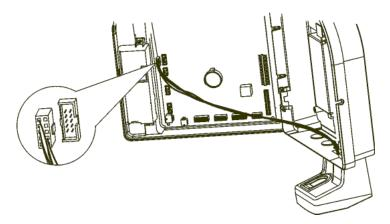
b. Disconnect the green ground wire leading from the verification device by removing the screw and freeing the wire. Then, reinstall the screw.
