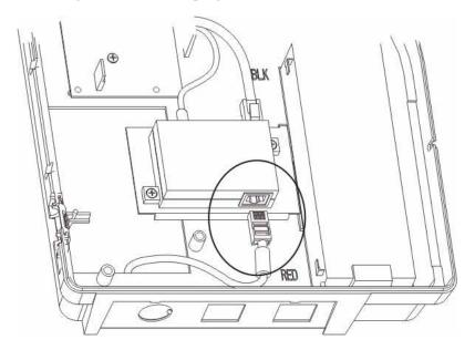
If the device uses the *GT-91080 Power-over-Ethernet module* (beige module), refer to the following illustration to unplug the Ethernet cable from the module:
