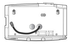
**Warning:** If the Ethernet cable is also the source of power for the device, do not plug it into the main board until you are directed to do so.
