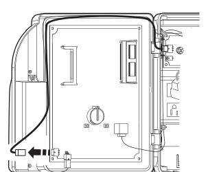
connector at the end of the cable and pull it to the left while moving the connector from side to side
