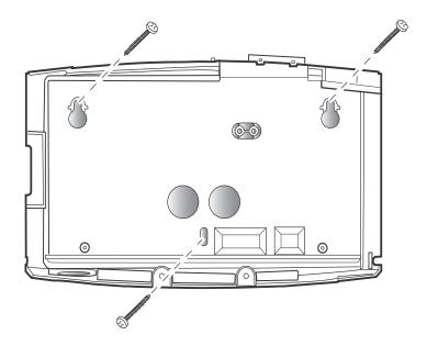
3. Tighten the top two screws and bottom middle screw so that they are flush against the base of the Kronos  $InTouch^{TM}$ .
