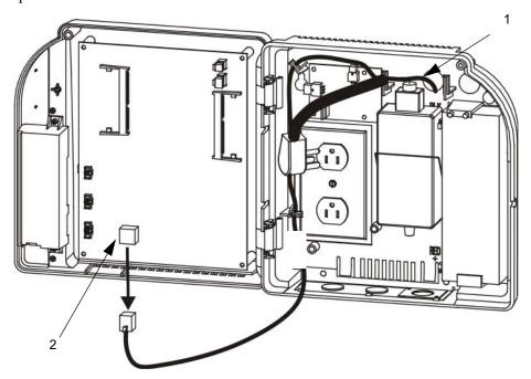
If the part number of the device is 8602000-xxx, use the following illustration to locate the Ethernet cable (1) and the connector on the main board (2). Then, press the clip on the connector and pull it down.
