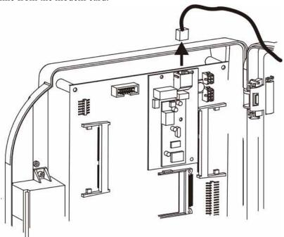
For devices that use *Ethernet communication*, disconnect the Ethernet cable (1) from the connector (2) on the main board. Press the clip on the connector and pull it down.
