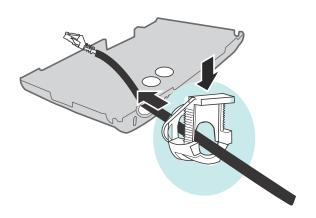
3. Push the clip assembly through hole in the base
