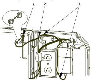
If the part number of the device is 8602000-xxx, use the following illustration as a guide. The numbered arrows point to the transformer cable (1), molded hooks (2), and the transformer connection on the main board (3).
