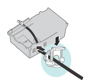
3. Push the clip assembly through hole in the base.
