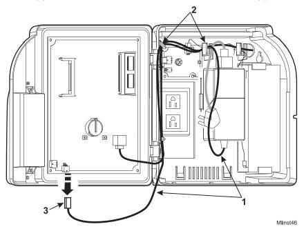
7. Unplug the power cable from the top of the transformer in the base of the device. See the circled area in the following illustration:
