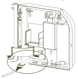
14. Disconnect the end of the ribbon cable that connects the interface board to the main board in the cover (circled in the following illustration).
