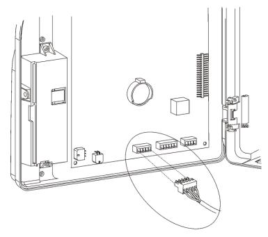
12. If your device uses a universal relay (for example, to ring a bell or operate a door strike), disconnect the relay from the device main board and thread the cable out of the device.
