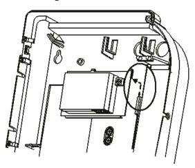
4. Determine whether the device has a backup battery (1) installed in the base. If so, go to step 5. Otherwise, go to step 6.
