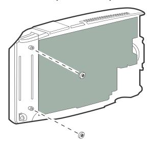
5. Insert the reader cover back onto the base. Tighten the screws on the reader cover.
