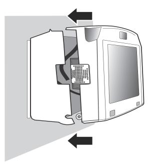
2. Use the security wrench to tighten the top screw and then the two screws on the sides.
