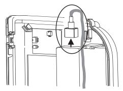
8. This step explains how to disconnect the modem or Ethernet cable, depending on which method of communication the device uses.
