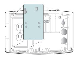
2. Using the two large holes on the right that you marked on the wall from the mounting template or the base, use a 3/8 inch drill bit to drill holes into the wall at those marked locations. Those holes will be used to run the Ethernet cable, the cable from a remote reader, and any other cables that you plan to run through the wall in to the base of the Kronos InTouch<sup>TM</sup>.
