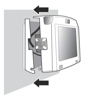
2. Use the security wrench to tighten the top screw and then the two screws on the sides.
