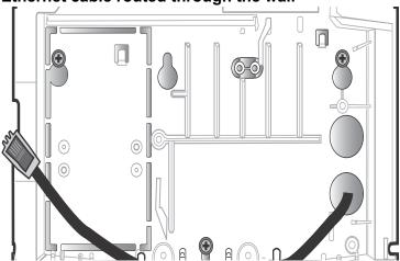
Ethernet cable routed through the bottom of the base
