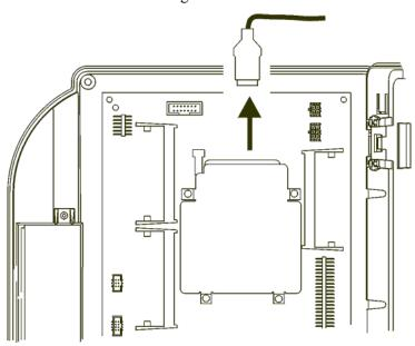
*If the part number of the device is 8602800-xxx*, use the following illustration to locate the modem card in the inside cover. Then, disconnect the telephone line from the modem card.
