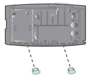
**Note:** To install with the direct AC wiring option, you must use the bottom hole on the left side of the base (right side in the view from the back in the illustration above). See "Example 2: Mounting with direct AC wiring" on page 36. Use the other holes to run other cables.
