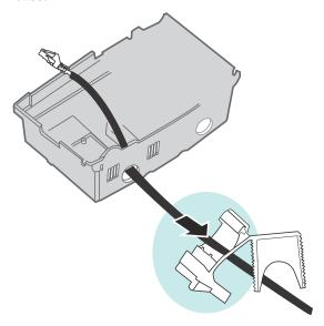
2. Close the top and bottom halves of the clip together and then insert that assembly through the hole in the base.
