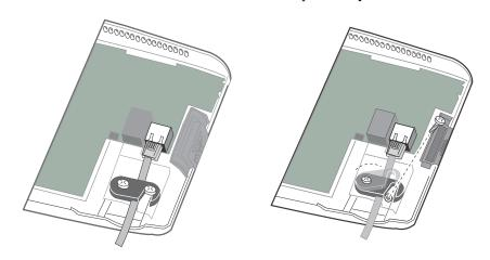
2. Push in the top of the Ethernet connector clip and then pull out the cable.
