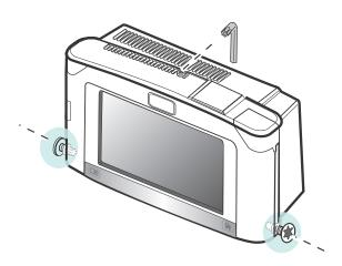
2. Open the cover *slowly* and *carefully*. You may not be able to open the cover all the way if there are cables from optional components connected to the main board.
