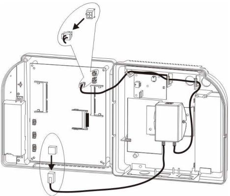
b. Grip the power-over-Ethernet module firmly and push up so that the module and its mounting bracket slide off the channels molded into the
