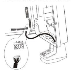
If the part number of the device is 8602000-xxx, use the following illustration to locate the connection. Then, unplug the verification device from its connection on the main board.
