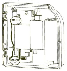
b. Disconnect the remote proximity reader from the connection on the interface board, as shown in the following illustration:
