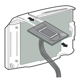
2. Remove the screws and then unplug the board from the main board.
