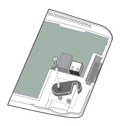
b. Swivel the clip over the Ethernet cable.
