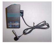
The Digital Wireless Audio DSS system is a digital frequency-agile radio designed to achieve excellent audio recording for the various Eyewitness Video systems.
