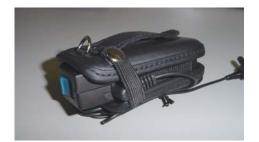
The transceiver can be used with or without the supplied mic cord. There is an internal mic on the transceiver that will be used if you do not use the cord, or if the cord becomes damaged. For best results, we recommend you use the cord. When you plug it in, route the cord downward as shown, so the strap will hold the plug securely in place.
