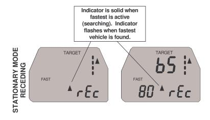
To place the unit in the stationary mode, monitoring receding traffic, repeatedly depress the MODE switch until "rEc" is displayed in the PATROL window.
