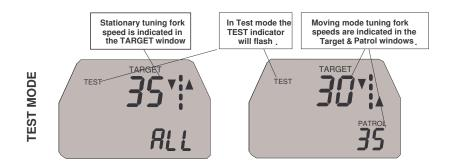
Pressing the TEST button places the radar in **test** mode, which is indicated by the flashing TEST indicator. While in test mode, the radar will display all speeds, both moving targets and non-moving targets such as tuning forks. The unit will remain in test mode for 30 seconds. Selecting a new mode, such as changing from stationary to moving, will refresh the timeout to 30 seconds allowing fork testing of all modes.
