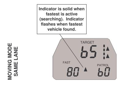
When operating the radar in Same-Direction mode, the same direction road indicator corresponding to the antenna selected will be on solid, and the strongest vehicle speed will be displayed in the TARGET window.
