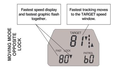
If the Lock button is pressed while tracking a fastest vehicle in any mode, the fastest speed will be locked in the LOCK window, and the fastest tracking will move to the TARGET window. After lock, both the LOCK window and the fastest indicator will flash together.
