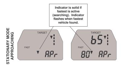
To activate the stationary, approaching targets only mode, repeatedly depress the MODE switch until "APr" appears in the PATROL window.
