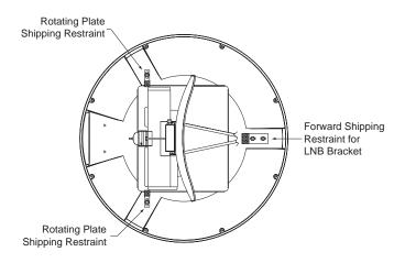
13. For convenient storage, rotate the shipping restraints 180° and secure them to their original mounting bolts using the nuts and washers removed in Step 12 (see Figures 2-8 through 2-10). All nuts and washers removed in Step 12 must be reinstalled. These nuts and washers secure the baseplate to the mounting plates.
