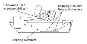
12. Remove the nuts and washers securing the shipping restraints to the baseplate. The positions of all three shipping restraints are pictured in Figure 2-7.
