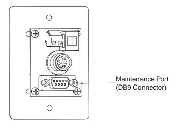
2. Connect the other end of the PC data cable to the serial port on the PC (a 9-pin/25-pin connector adapter may be needed for some PCs).
