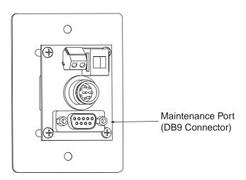
2. Connect the other end of the PC data cable to the serial port on the PC (a 9-pin/25-pin connector adapter may be needed for some PCs).
