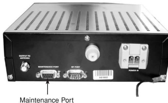
Figure 4-3 MCU Maintenance Port
