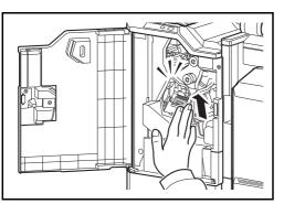
4 Close the cover (A) plate of the staple cartridge holder into its original position.
