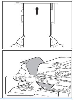
After printing starts, catch the paper when it is output so that it does not fall.When using the inner tray as the output location, do not stand up the stopper. Standing up the stopper may cause paper jams.
