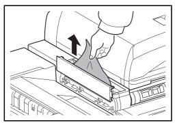
4 Turn the conveyor knob (D3) to the left to feed the paper along to enable easy removal.
