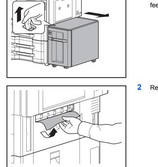
1 Pull up the release lever and separate the side feeder from the multifunction machine.
