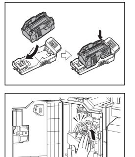
4 Insert the new staple cartridge into the staple cartridge holder.
