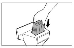
Insert the key counter securely into the key counter slot.
