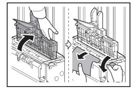
1 Lift up the folding tray and remove any jammed paper.
