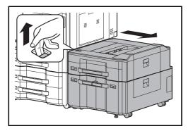
1 Pull up the release lever and separate the side feeder from the multifunction machine.
