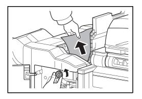
5 Turn the conveyor knob to the left to feed the paper along to enable easy removal.
