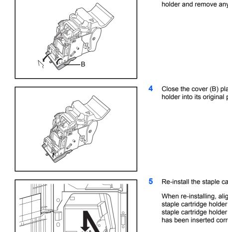
3 Open the cover plate (B) of the staple cartridge holder and remove any jammed staples.
