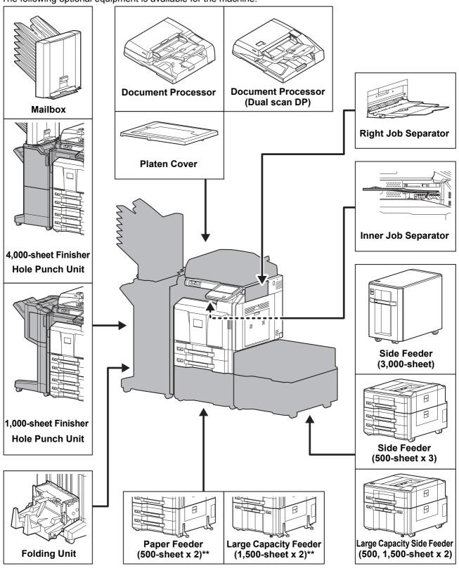
\* The side feeder (500-sheet x 3) or large capacity side feeder (500, 1,500-sheet x 2) can be used on a 45/45 ppm model or a 55/50 ppm model.
