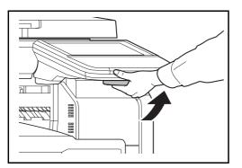
Adjust the angle of the operation panel in two as shown by releasing the operation panel lock lever.
