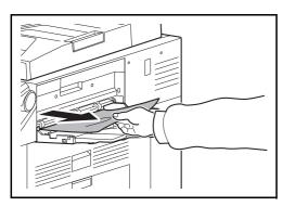
1 If jammed paper is seen through the paper ejection slot of the right job separator, pull it toward your side to remove it.
