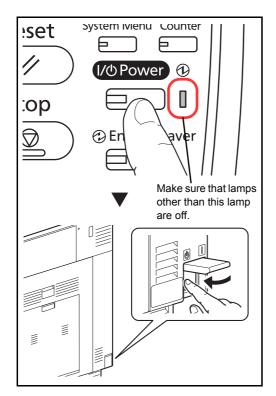
1 When the machine is powered up, first press the **Power** key on the operation panel. Check that the **Power** indicator, the processing indicator and the memory indicator are off. After this, turn off the main power switch.
