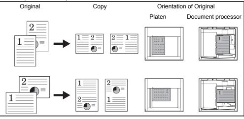
**NOTE:** When placing the original on the platen, be sure to copy the originals in page order.
