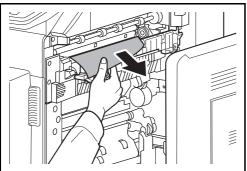
1 If jammed paper is seen through the paper ejection slot of the inner job separator, pull it toward your side to remove it.
