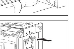
5 If jammed paper is seen through the paper ejection slot, pull it toward your side to remove it.
