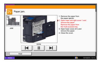
If a paper jam occurs, the touch panel will display *Paper Jam.* and the machine will stop. Refer to these procedures to remove the jammed paper.
