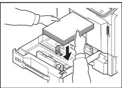
3 Press the (Paper Width Guide) Lock to release the lock. Grasp the paper width adjusting tab and move the paper width guides to fit the paper.
