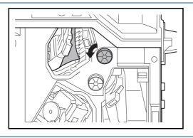
**NOTE:** If it is difficult to remove the jammed paper, turn feed knob D3 until the jammed paper is in a location where it is easy to remove.
