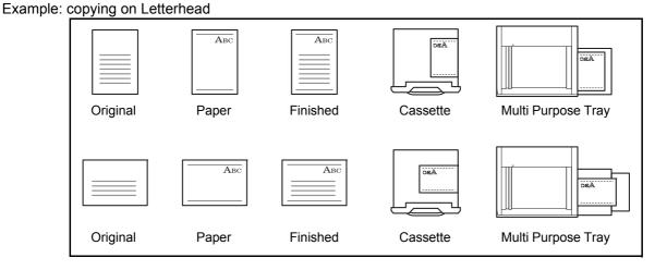
**NOTE:** When loading cover paper in a cassette or multi purpose tray, load the face, on which printing is supposed to be done, upward.
