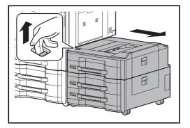
1 If you are using the optional side feeder, pull up the release lever and separate the side feeder from the multifunction machine.
