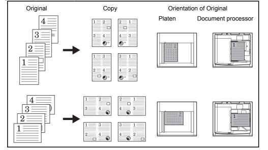
NOTE: When placing the original on the platen, be sure to copy the originals in page order.
