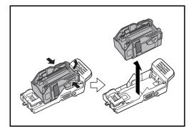
3 Remove the empty staple cartridge from the staple cartridge holder.
