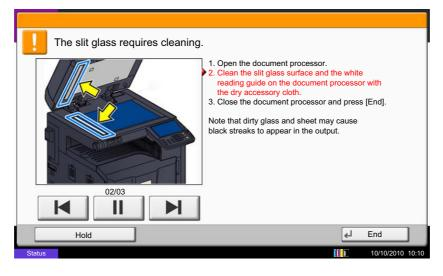
**NOTE:** Wipe the slit glasses with the dry accessory cloth. Do not use water, soap or solvents for cleaning.
