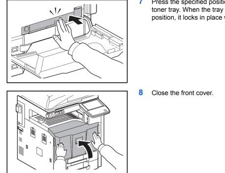
7 Press the specified position to close the waste toner tray. When the tray reaches the correct position, it locks in place with a clicking sound.
