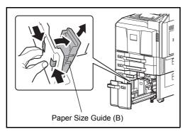
4 With the bottom of the cassette pressed all the way down, press the hook on the side of the Paper Size Guide (B) to release it and pull out the Paper Size Guide (B).
