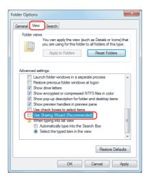
In Windows XP, click the View tab and remove the checkmark from Use Simple File Sharing (Recommended) in Advanced settings.
