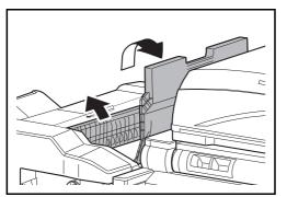
1 If jammed paper is seen through the paper ejection slot, pull it toward your side to remove it.
