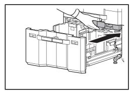
8 Open the paper feed unit cover (B2) and remove the jammed paper.
