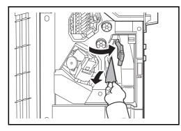
1 If jammed paper is seen through the paper ejection slot, pull it toward your side to remove it.
