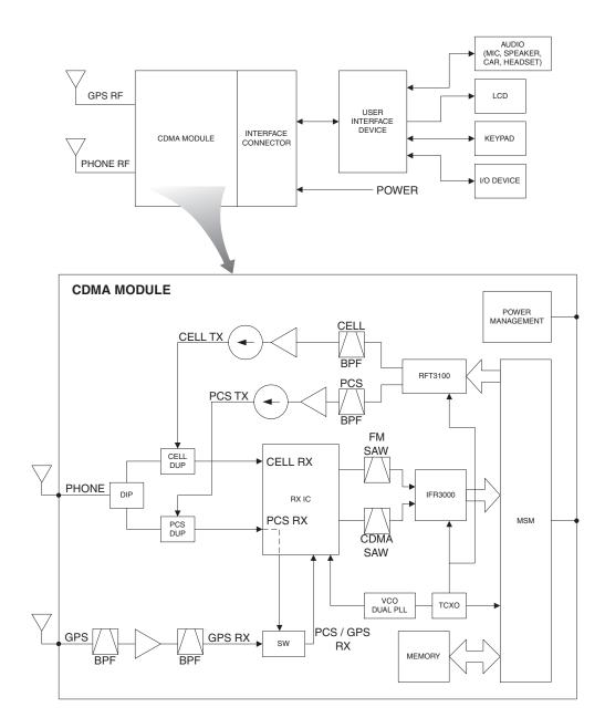
The Module card includes the following circuits, with the necessary filtering and AGC circuits to meet performance requirements.
