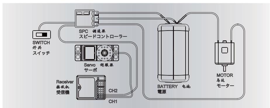
**Remark:** to guarantee a long range, place the antenna of the receiver vertically away from any metal part.
