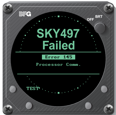
Figure 2-5. SKY497 Failed Screen
