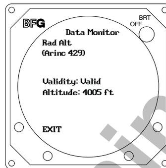
If DC Analog Radio Altimeter was selected in equipment menu the following data monitor will appear:
