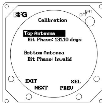
After a successful calibration, the new Bit Phase value will be displayed.
