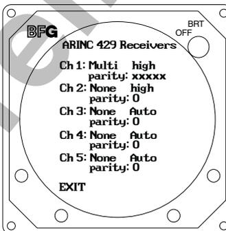
Parity display is the count of bad parities received. If the number is continuing to increase that is typically a sign of bad data being received.
