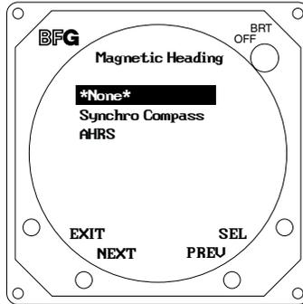
Selecting Synchro Compass causes Heading Valid Line menu to appear:
