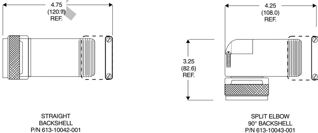
**Figure 1-5. P1 Connector Dimensions (Reference Only)**
