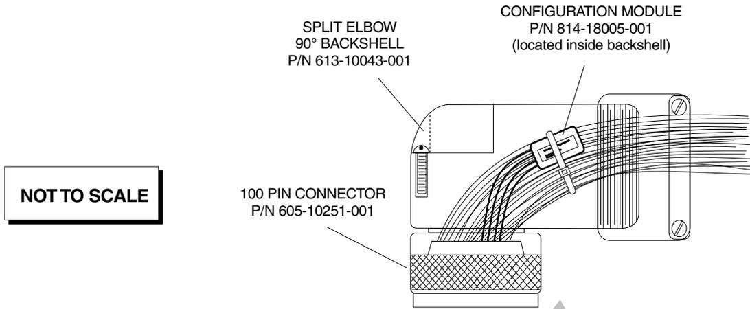
**Figure 2-9. Typical Location of System Configuration Module (Inside Backshell)**
