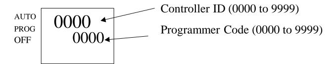
Controller ID- Every controller must have a unique ID. This will prevent a conflict if more than one controller is within range of the radio signal. Write down the Controller ID for future reference. Warning: Do not select the same Controller ID for two controllers within 1 mile of each other. Improper radio operation may result.
