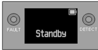
Full Battery in Standby Mode
