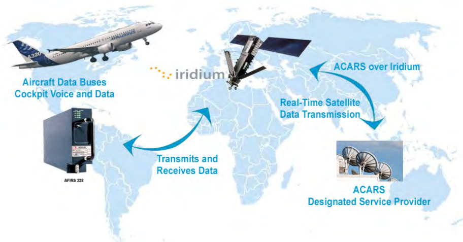
Figure 2-1 –Iridium SATCOM System Operational Concept
