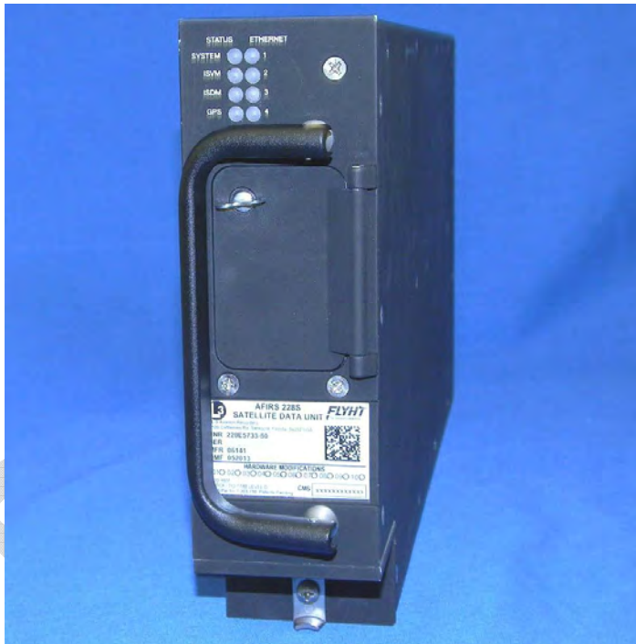
Figure 3-1 –Iridium SATCOM System Satellite Data Unit (SDU)
