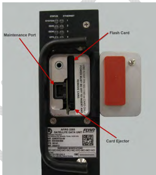
Figure 7-1 – Maintenance Port Location
