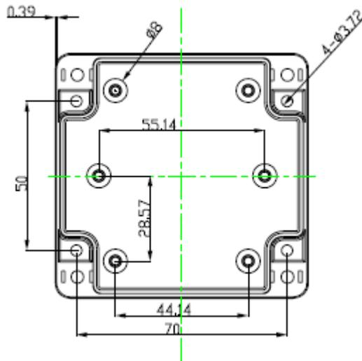
**Figure 3. Screw mounting holes for outdoor fixture**
