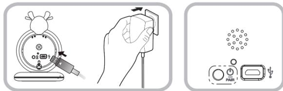
C. Connecting the power supply for the Parent Unit.
