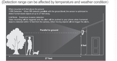
PIR sensing zone is divided into two 120° sectors: left and right, they can be switched on and off independently. As shown in the following picture.
