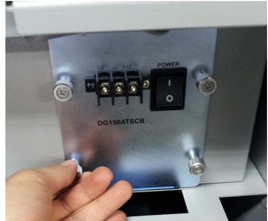
② Unfasten fixed screw which is connecting to exterior and pull forward.
