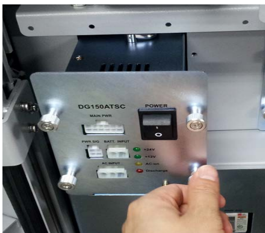
② Unfasten fixed screw which is connecting to exterior and pull forward.
