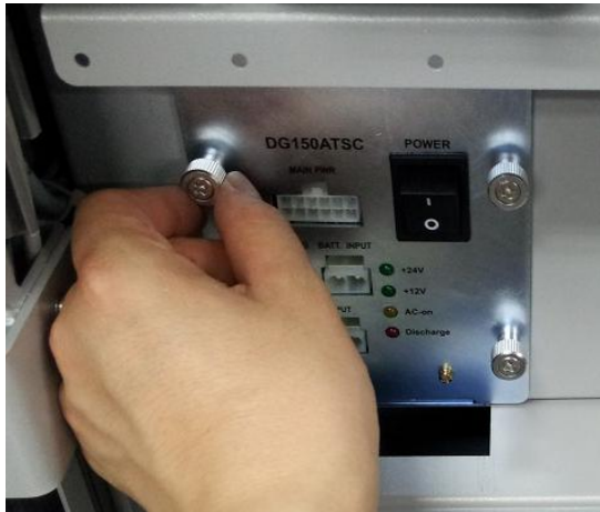
② Unfasten fixed screw which is connecting to exterior and pull forward.
