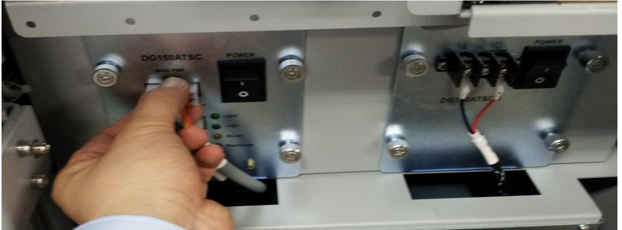
① Separate Connector which is connecting SMPS and Battery.
