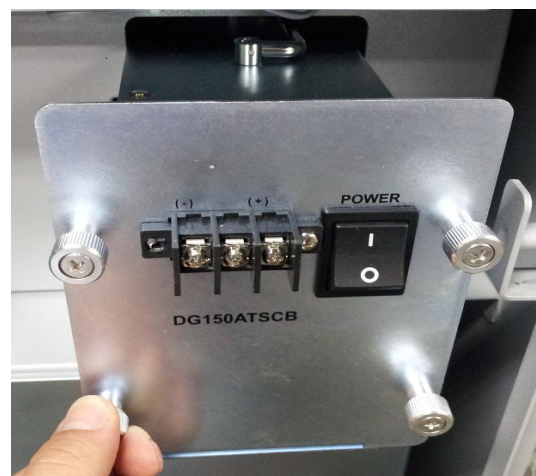
② Unfasten fixed screw which is connecting to exterior and pull forward.
