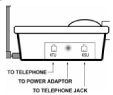
3 Plug the modular cable supplied with your new Wanderer into the charging base jack labeled KTU. Plug the other end of this cable into your existing wired telephone.
