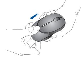
**English** At the buttom of the mouse, follow the direction of the arrow to push gently, at the same time, to pull out the battery cover in opposite direction, to pull out the battery
