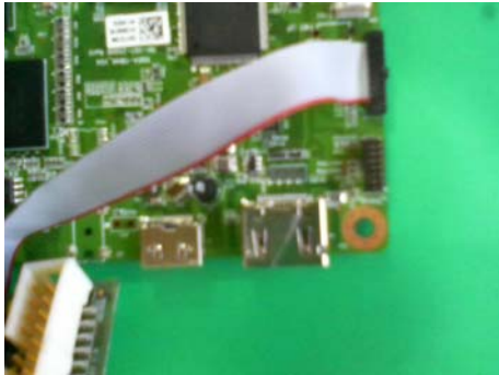
Figure 7: UART Cable connection Method
