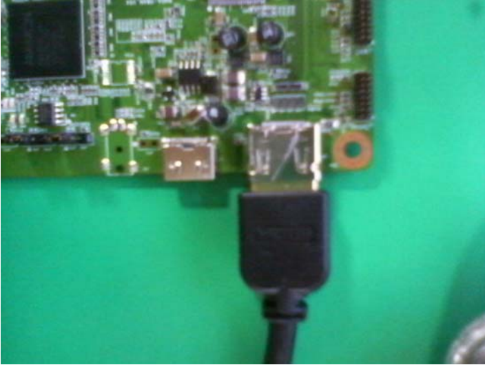
Figure 4: HDMI Cable connection Method
