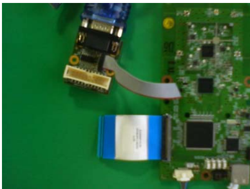
Figure 7: UART Cable connection Method
