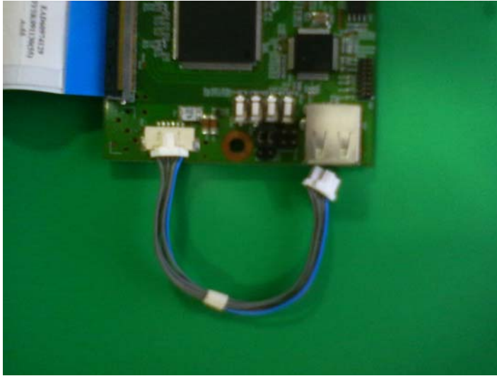
Figure 4: Power Cable connection Method
