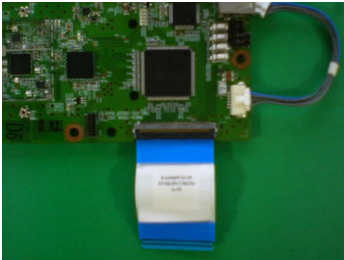
Figure 3: A/V and Control Cable connection Method
