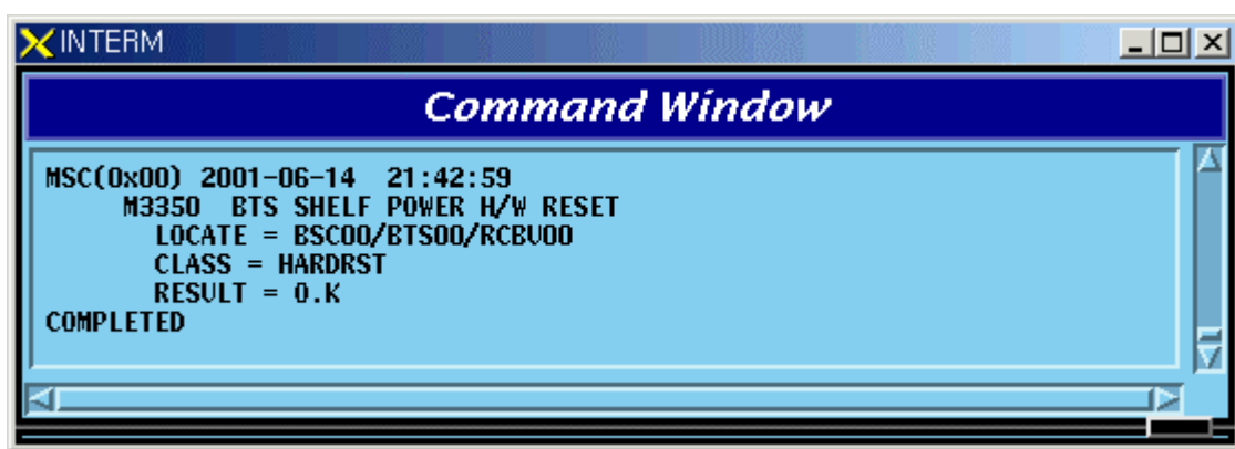
Fig. 4.4-41 Result of BTS SHELF POWER H/W RESET Command
