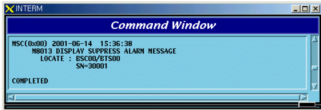
Fig. 4.8-6 Display Result of Display Command for the Suppressed Alarm Message
