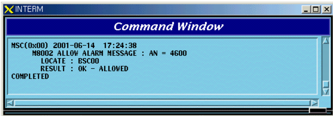
Fig. 4.8-15 Display Result of Allowance for Alarm Message Display Inhibition
