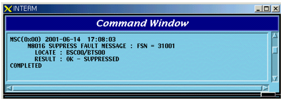
Fig. 4.8-19 Display Result of Release Command for Suppressed Fault Message
