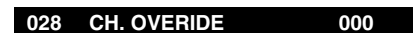
After Master TV setup has been completed, set item 028 Ch Override to 000.
