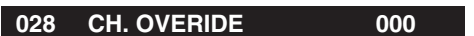
After Master TV setup has been completed, set item 028 Ch Override to 000.
