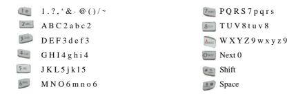
After a character is entered, the cursor automatically advances to the next space after two seconds. You can also advance the cursor by pressing for entering a character not on the same key.
