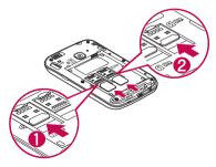
3 Insert the battery into place by aligning the gold contacts on the phone and the battery (1) and pressing it down until it clicks into place (2).
