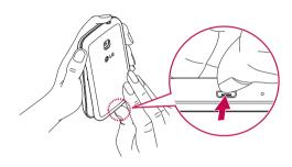
2 Slide the SIM card into its slots as shown in the figure. Make sure the gold contact area on the card is facing downwards.
