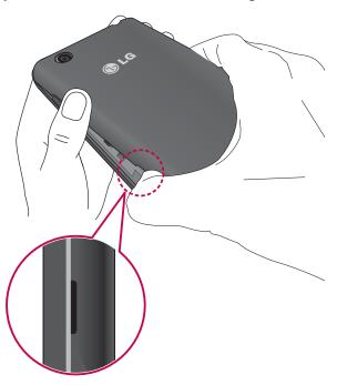
2 Slide the SIM card into its slot as shown in the figure. Make sure the gold contact area on the card is facing downwards.
