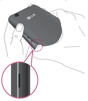
2 Slide the SIM card into its slots as shown in the figure. Make sure the gold contact area on the card is facing downwards.
