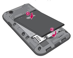
4 Align the back cover over the battery compartment (1) and press it down until it clicks into place (2).
